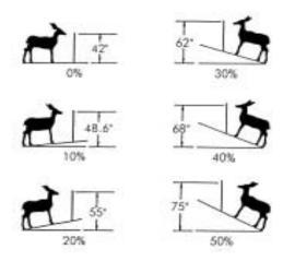
Barrier Height Increase of 42" Fence on Contour of Different Percent Slopes
